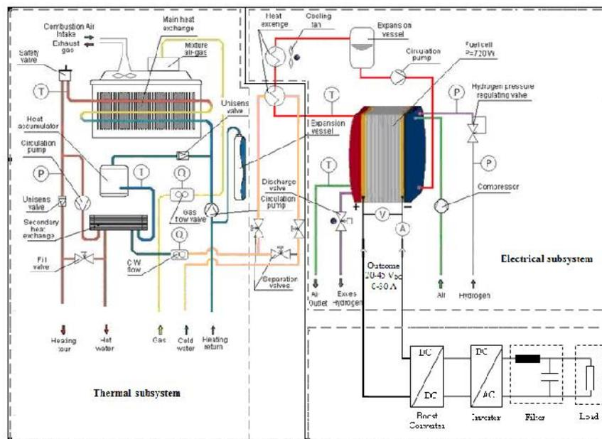
Figure 3 .The electrical and thermal schemes for the experimental energy system.
