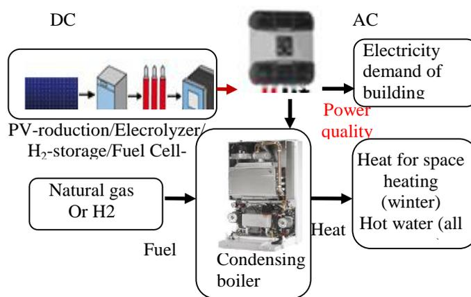
Figure 2. DER solution for the energy supply of boiler
