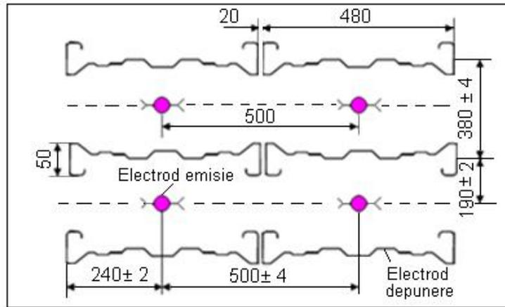
Figure 11. Model of layout of the deposit electrodes against the emission electrodes - variant 3
