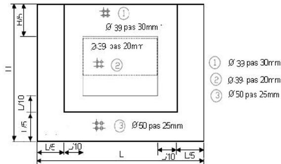
Figure 9. The levelling sieve S4
