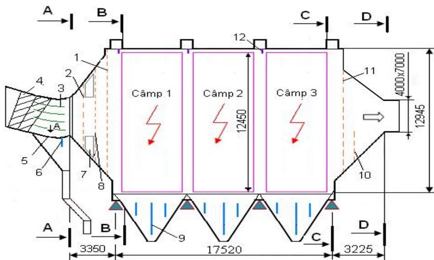
Figure 2. Electrostatic precipitator assembly – location of measurement sections
