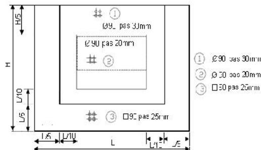
Figure 10. The levelling sieve S5
