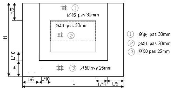
Figure 8. The levelling sieve S3
