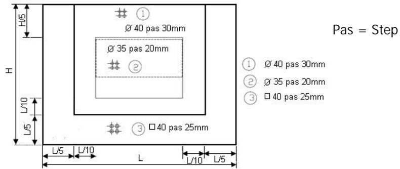
Figure 6. The levelling sieve S1
