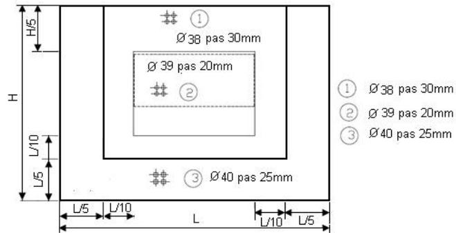
Figure 7. The levelling sieve S2
